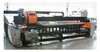
The application of ceramic frit coatings on the glass is carried out in the factory in a controlled environment. The ink layer is deposited on a flat surface of the glass using an inkjet printer and is then vitrified on this surface during the glass tempering process. A whole new technological advance in digital printing with a high-definition 4-color printing process plus black and white. The result is a solid, durable, stable and inert coating scratch, weather and UV resistant.
