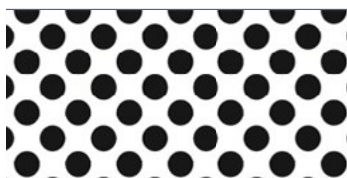
G009 Dots 3mm (1/8") diameter Spaced 6mm (1/4") Centre to centre 40% Coverage
