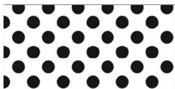
G008 Dots 3mm (1/8") diameter Spaced 7mm (9/32") apart Centre to centre 30% Coverage
